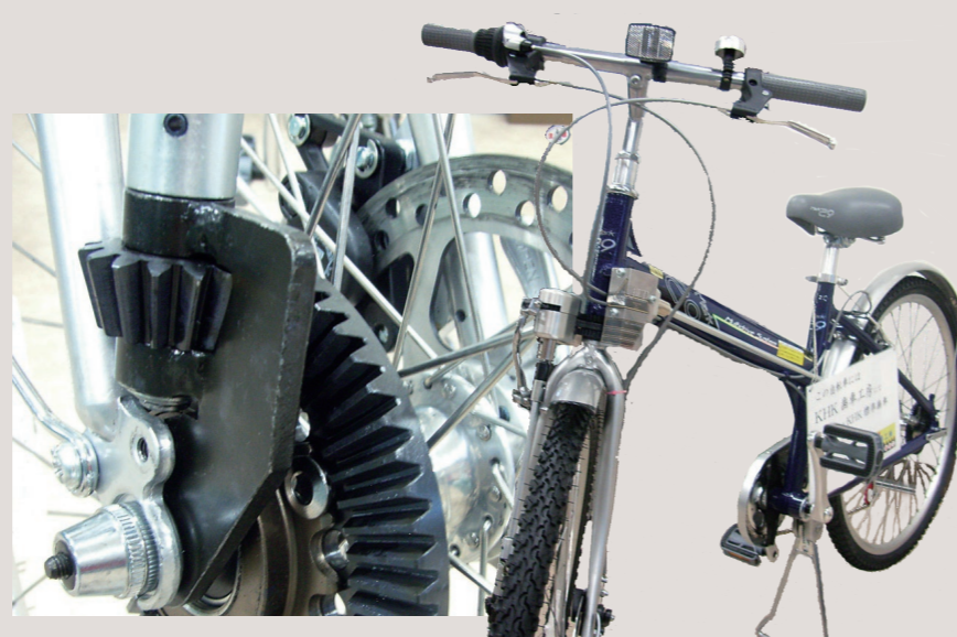
KSB Bevel Gears are used in the driving components in both the front and rear wheels
